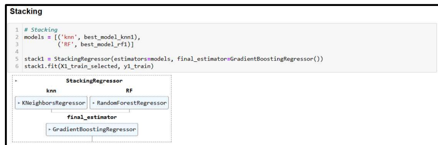
Figure 13. Stacking Method for Improvement of Model
